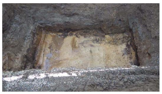
Photo 23: View into TN36;-12 with PVC pipe and drain rock visible near surface.
