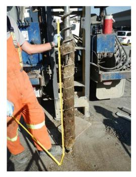
Photograph 8: Auger flight from BH17- 58 (0 to 150 cm DBS), looking northwest.
