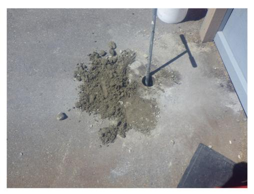
Photograph 1: Example of hand auger test (HA17-41) in progress, looking south.
