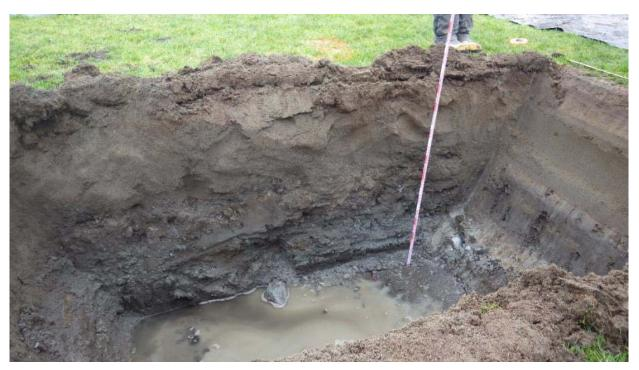
Photo 11: View west into TN41;-80, with a possible original land surface (with dark organics) under engineered sandy fill to a depth of about 60 cm.
