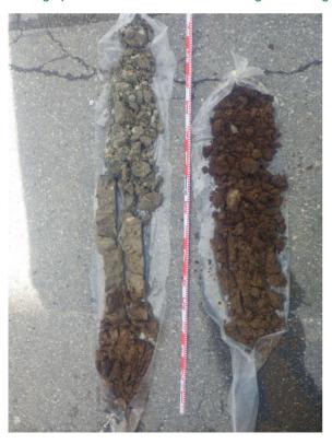
Photograph 6: Recovered samples from sonic drilling of BH17-30 (1.5 m to 3 m DBS on the left and 0.30 to 1.5 m DBS).
