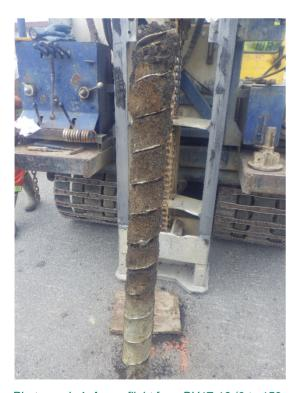
Photograph 4: Auger flight from BH17-16 (0 to 150 cm DBS), looking northwest.
