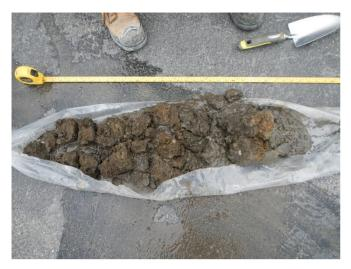
Photograph 9: Recovered samples from sonic drilling of BH17-63 (0 m to 1.5 m DBS).
