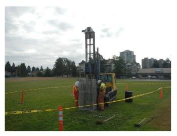
Photograph 7: General view of solid stem auger rig conducting borehole test (BH17-51). Looking east.
