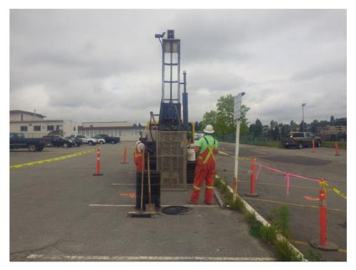
Photograph 3: General view of solid stem auger rig conducting borehole test (BH17-16). Looking northwest.
